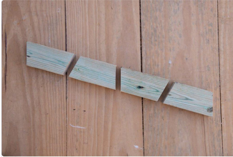
Fig. 3. Four gussets cut from the remaining board. Photo: The Home Depot.
