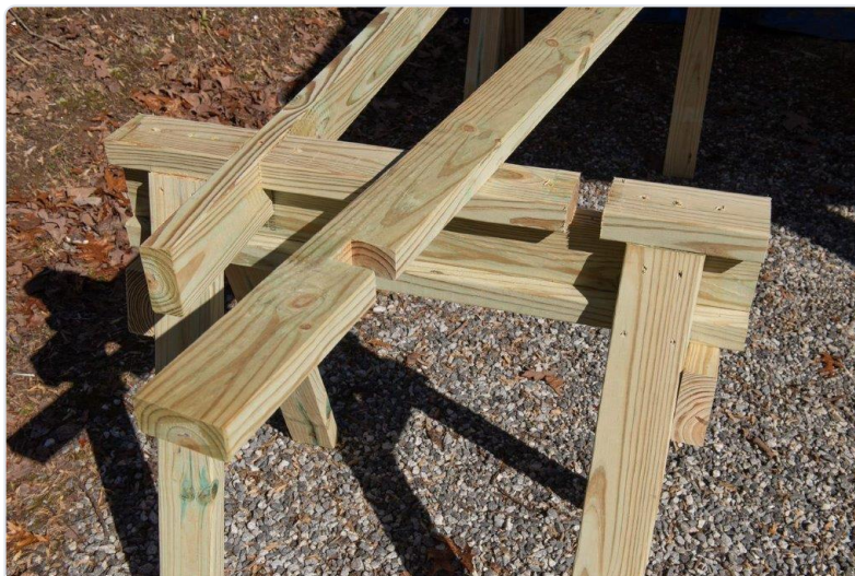
Fig. 8. Finished sawhorse with notches cut for a tabletop. Photo: The Home Depot.
