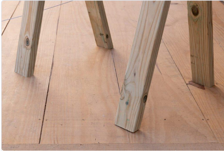
Fig. 6. Standing the sawhorse up and checking for balance. Photo: The Home Depot.
